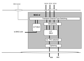
Note 1: For DCH and DSCH different scheduling mechanism apply Note 2: Ciphering is performed in MAC-d only for transparent RLC mode
